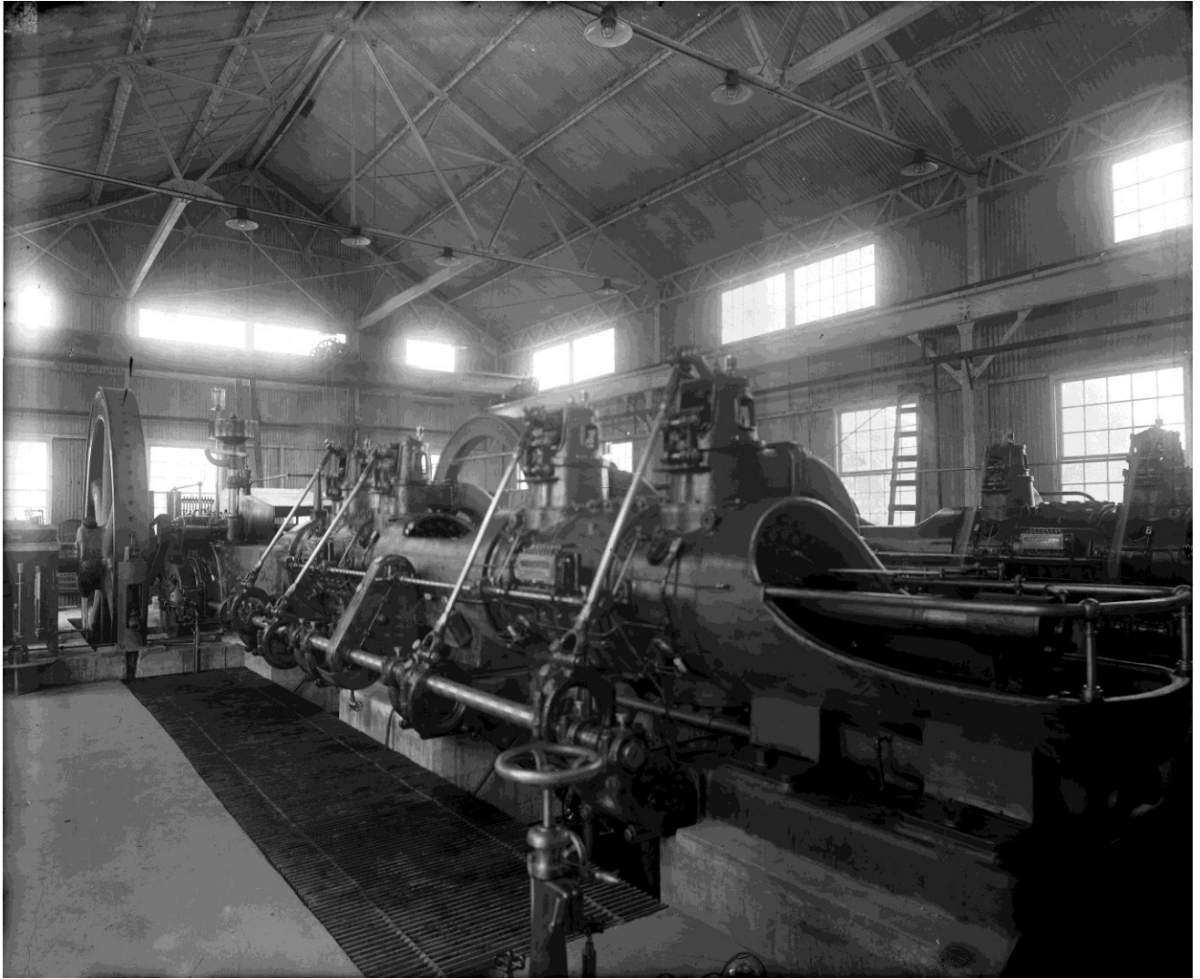
Picture from a glass negative of two Coopers in a compressor station, location unknown.
